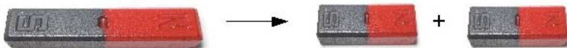
A bar magnet (left) and the result of chopping it in half (right).
